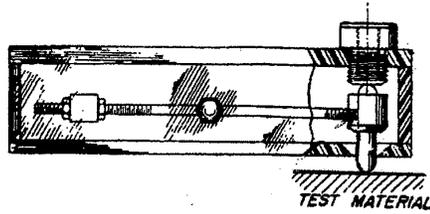
PERMEABILITY VALUE OF TEST MATERIAL IS HIGHER THAN THAT OF INSERT (MAGNET REMAINS IN CONTACT WITH TEST MATERIAL)
